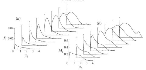
FIGURE 20. (a) Turbulent kinetic energy K, (b) turbulent Mach number  $M_t$  at downstream stations 2–9, according to figure 2.
