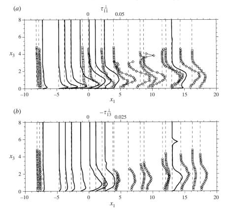
FIGURE 18. Downstream evolution of Reynolds-stress profiles: (a)  $\tau_{11}^{\perp}$ , (b)  $-\tau_{13}^{\perp}$ ; —, simulation data;  $\Box$ , ExpB;  $\diamondsuit$ , ExpC; thin dotted vertical lines are the reference lines for the respective profiles, which give the downstream position  $x_1$  from the ramp corner (lower horizontal axis) and from which the magnitude of  $\tau^{\perp}$  is measured (upper horizontal axis).
