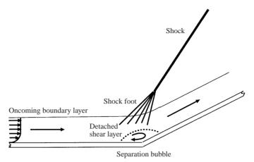
FIGURE 1. Sketch of the compression-ramp configuration.
