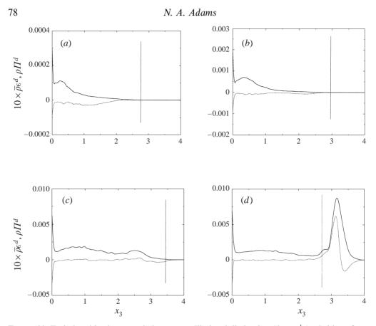
FIGURE 22. Turbulent kinetic energy balance, —, dilational dissipation  $10 \times \bar{\rho} \varepsilon^d$  (scaled by a factor of 10); ....., pressure dilatation  $\bar{\rho}\Pi^d$ ; (a) station 2, (b) station 4, (c) station 7, (d) station 9; the vertical solid line indicates the 99% local mean boundary-layer thickness.
