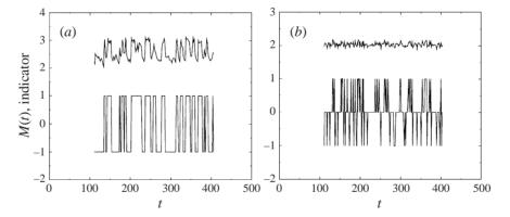
FIGURE 14. (a) Mach-number traces and shock indicator at  $x_1 = 44.88$  and  $x_3 = 7.76$ , (b) Mach-number traces and burst indicator at  $x_1 = 8.62$  and  $x_3 = 1.27$ .
