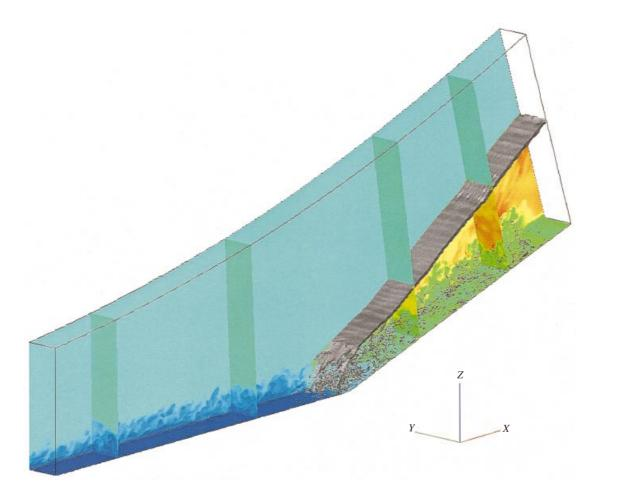
FIGURE 11. Density at the wall, in the plane  $x_2 = 2.9$  and 4 crossflow planes; shock-surface with  $\partial_{x_i} u_i = -0.4$ ; high density: red; low density: blue; solid black lines indicate the computational-domain boundaries.
