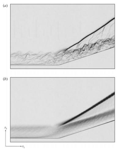
FIGURE 9. Flow-field Schlieren imitation,  $||\nabla \rho||$  contours, (a) instantaneous  $x_2$ -average, (b)  $x_2$ -average and time average using 100 samples.
