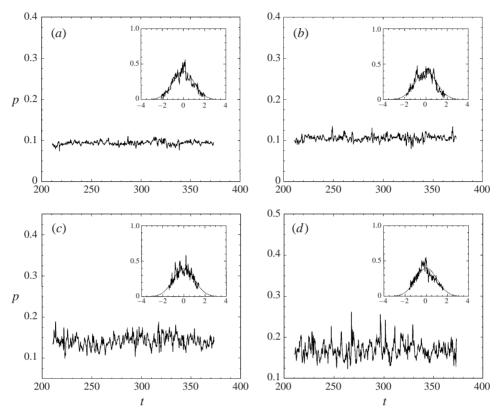
FIGURE 13. Wall-pressure traces at positions (a)  $x_1 = 31.6$ , (b)  $x_1 = 32.8$ , (c)  $x_1 = 35.0$ , (d)  $x_1 = 36.4$ , in the plane  $x_2 = 0$ ; normalized PDF in inset, dotted line is a Gaussian distribution, for reference.
