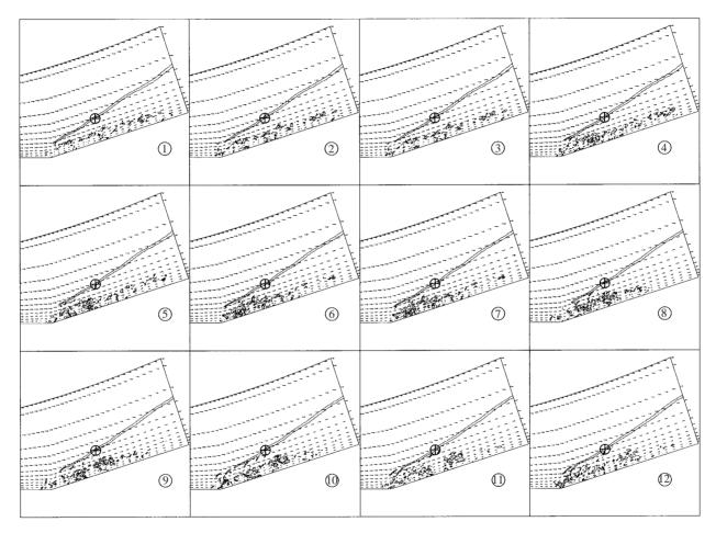
FIGURE 12. Sequence of shock evolution (iso-contours of  $||\nabla p||$ ) and velocity vectors at  $x_2 = 0.72$  for a sequence of equal timesteps between  $t_l = 309.00$  and  $t_r = 325.34$ ; sequence from bottom to top and left to right (numbers 1 to 12); the marker indicates the sensor position for figure 14; flow direction is from bottom up.
