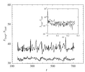
FIGURE 15. Time trace of spanwise-averaged separation and reattachment line (as defined in the text), Fourier decomposition in the inset.
