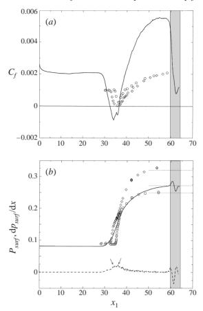
FIGURE 8. (a) —,  $C_f$  and (b) —,  $p_{surf}$ , also shown is - - ,  $dp_{surf}/dx$ ; grey shaded area indicates the sponge region, arrows indicate first and last inflection point of  $p_{surf}$ ; O, experimental results ExpB;  $\diamond$ , experimental results ExpC.
