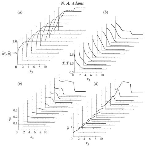
FIGURE 5. (a) Alternating — and - - - for  $\tilde{u}_1^c$  (thick lines) and for  $\bar{u}_1^c$  (thin lines); (b) —,  $\tilde{T}$  (thick lines) and —,  $\bar{T}$  (thin lines); (c)  $\bar{p}$ , and (d)  $\bar{\rho}$  at downstream stations 1–10 according to figure 2. Note that in (a) and (b) although two lines (thick and thin) are shown at each station, they mostly overlap and are indistinguishable.
