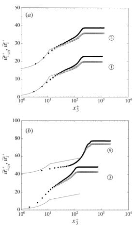
FIGURE 7. Contravariant-velocity profiles scaled in wall units; (a) at stations 1 and 2, bottom-up; (b) at stations 3 and 9 bottom-up;  $\bigcirc$ ,  $\bar{u}_1^{c^+}$ ;  $\bigcirc$ ,  $\bar{u}_{1_{VD}}^{c^+}$ ; -----, law of the wall  $x_3^+$  and  $(2.5 \ln (x_3^+) + 5.5)$ ; for clarity staggered by 15 and 40, respectively.
