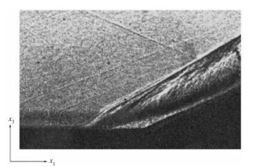
FIGURE 10. Flow-field experimental Schlieren visualization of a 25° compression ramp at  $M_{\infty} = 2.9$ ,  $Re_{\theta} = 9600$ , provided by A. Zheltovodov, ITAM, Novosibirsk.
