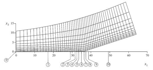
FIGURE 2. Computational mesh (each 20th line); numbers in circles indicate stations where profiles are shown in § 3.
