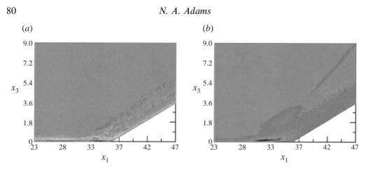
FIGURE 24. (a) Stretching production term  $\overline{I}_2$ , (b) baroclinic production term  $\overline{II}_2$ ; 8 grey-scale levels in the range  $-0.03 \leq \overline{II} \leq 0.06$  (light to dark).
