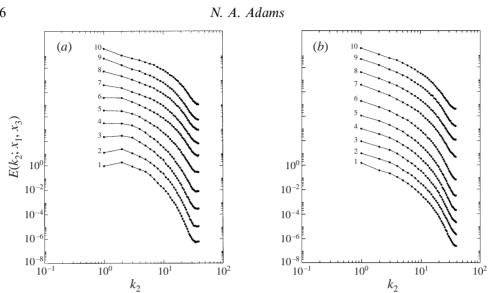
FIGURE 3.  $E(k_2; x_1, x_3)$  at downstream positions 1–10 (bottom-up), and (a)  $x_3^+ = 5$ , (b)  $x_3^+ = 97$  with respect to inflow; spectra are shifted by a factor of 10 for clarity.
