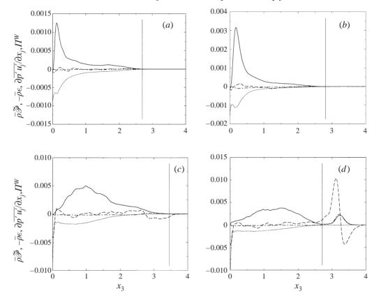
FIGURE 21. Turbulent kinetic energy balance, —, production  $\bar{\rho}\tilde{\mathscr{P}}$ ; ....., turbulent dissipation  $\bar{\rho}\varepsilon$ ; ----, pressure diffusion  $\partial \overline{p'u_j}/\partial x_j$ ; ---, pressure work  $\Pi^W$ ; (a) station 2, (b) station 4, (c) station 7, (d) station 9; the vertical solid line indicates the 99% local mean boundary-layer thickness.
